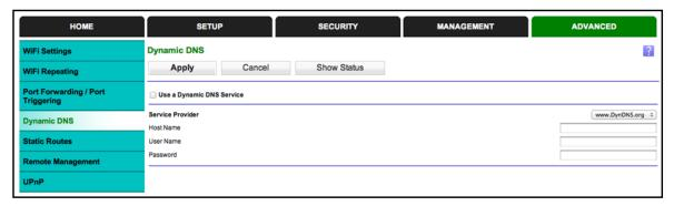
Figure 7. Forward traffic to a changing IP address
